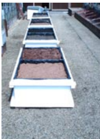
Plate 2.5 – Lysimeters filled with blends of composts and rock dust (1:1 v/v)
