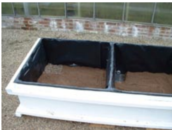
Plate 2.3 – Lysimeter for leachate collection with 10 cm sand.
